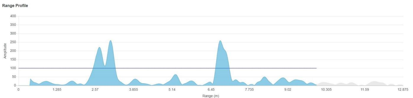
Given the previous section regarding radar noise, you can define what the sensor determines as noise and what it determines as a peak. This process of selecting peaks is conducted by tuning the "Target threshold" parameter in the Range Profile setting tab. Any graphical peaks above the target threshold are considered valid targets by the sensor and will trigger a sensor output if the peak is within the Range of Interest. The distinction between noise and peaks is presented in the figure above.
