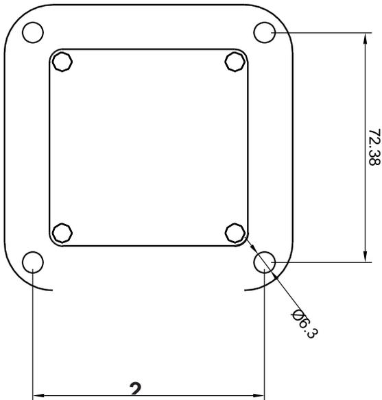
The sensor has a metal back facing the plane surface. It is recommended to mount the sensor on a metallic surface for best heat dissipation in hot environments.
