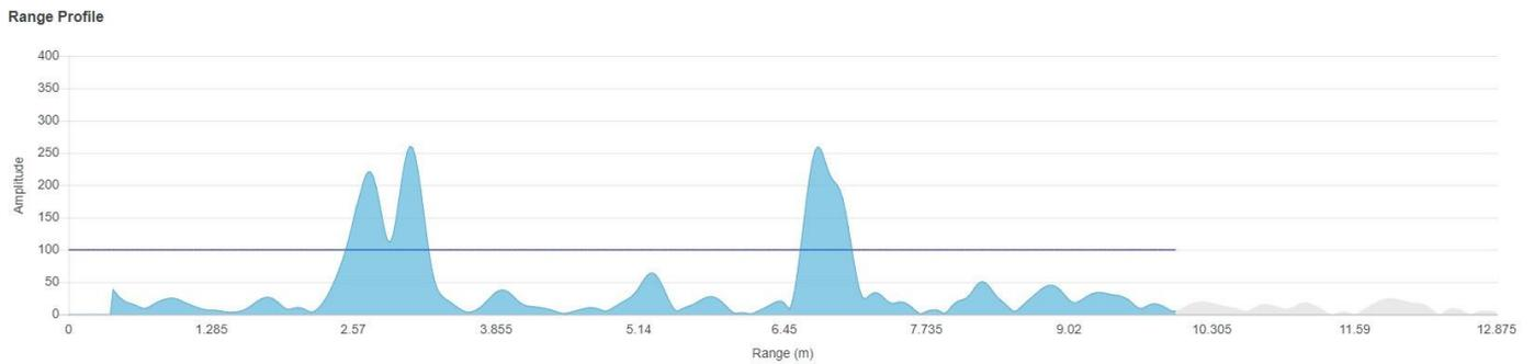
Range of Interest (RoI) is the delimited area within the Range Profile denoted in blue color. Everything outside the Range of Interest will have a faded grey color. Any targets within the RoI will generate an output, either pulling the relay, or sending a corresponding current on the current loop. The Range of Interest will not alter the accuracy or resolution of the radar.
