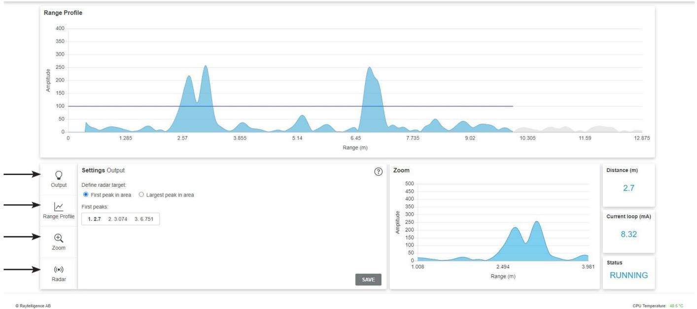
There are four different tabs to the left of the Dashboard used to decide the behavior of the radar and configure when the device should communicate to your end system. The four tabs are Output, Range Profile, Zoom, and Radar, described in more detail below.
